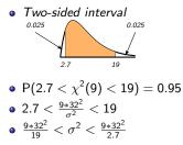
A container of oil is supposed to contain 1000 ml of oil. We want to be sure that the standard deviation of the oil container is less than 20 ml. We randomly select 10 cans of oil with a mean of 997 ml and a standard deviation of 32 ml. Using these sample construct a 95% confidence interval for the true value of sigma. Does the confidence interval suggest that the variation in oil containers is at an acceptable level?
